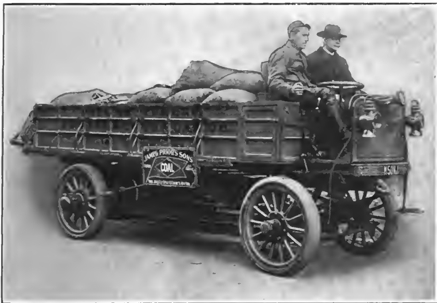
ATLAS THREE-TON GASOLINE TRUCK WITH ENGINE ON REAR AXLE.
